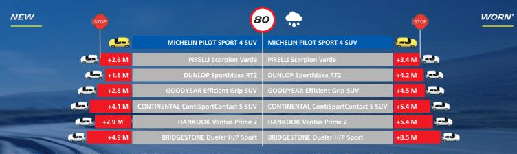
(2) Wet braking test, between 80 and 20 kph, conducted by TUV-SUD Product Service, on Michelin's request, in August 2018, on dimension 235/60 R 18 107W on Audi Q5 2.0 TDI \*\* Worm means worn on machine (birlifed) to the depth of Tad Wear Indicator FCF 830/03f
