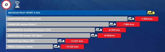
(3) Test conducted by DEKRA TEST CENTER, on Michelin's request, between August 2018 and September 2018, on dimension 235/60R18 107W on Hyundai Sante Fe CRDi. The longevity test runs in average real usage (D50) during 10,000km and an estimated longevity at 1.6mm.
